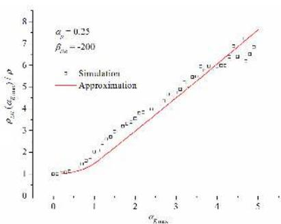
**Figure 11.** The resolution degradation of the multi-look SAP in the case of the harmonic error as the function of  $\alpha_{E\max}$  for  $\alpha_p = 0.25$ .
