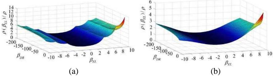
**Figure 5.** Degradation of the azimuth resolution versus the  $\beta_{EL}$  and  $\beta_{DR}$ , (a) for the rectangular window, and (b) for the Hamming window.
