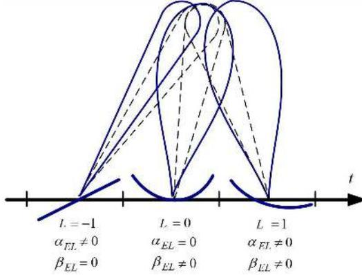
**Figure 1.** The influence of the local phase errors on SAR look beams.
