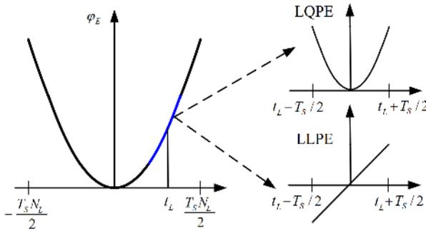
**Figure 7.** The quadratic phase error on the multi-look processing interval.
