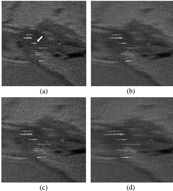
**Figure 14.** SAR images distorted by the quadratic phase errors introduced on the multi-look processing interval. (a) 15 looks,  $2 * \pi * \beta_p = 10$ . (b) 31 looks,  $2 * \pi * \beta_p = 10$ . (c) 15 looks,  $2 * \pi * \beta_p = 15$ . (d) 31 looks,  $2 * \pi * \beta_p = 15$ .
