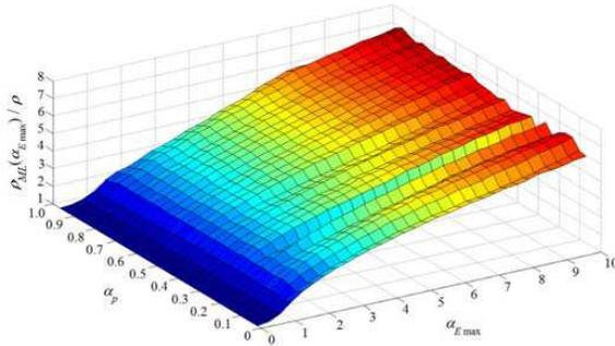
**Figure 10.** The resolution degradation of the multi-look SAP in the case of the harmonic error (numerical simulations).
