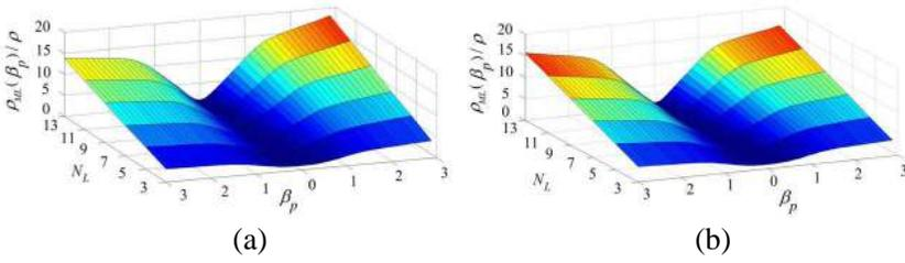
**Figure 9.** The degradation of the resolution of the multi-look SAP caused by the quadratic phase error on the multi-look processing interval versus the number of looks for the (a) low TBP and (b) high TBP cases.
