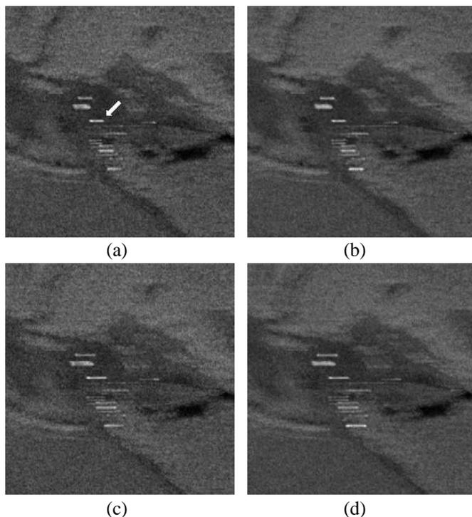
**Figure 15.** SAR images distorted by the harmonic phase errors with  $\alpha_p = 0.3$  introduced on the multi-look processing interval. (a) 15 looks,  $\beta_{E \max} = 10$ . (b) 31 looks,  $\beta_{E \max} = 10$ . (c) 15 looks,  $\beta_{E \max} = 15$ . (d) 31 looks,  $\beta_{E \max} = 15$ .
