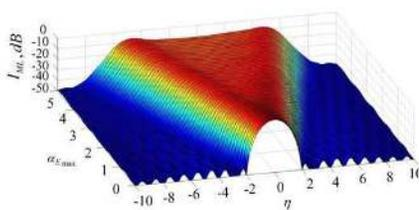
**Figure 12.** The multi-look SAP degradation in the case of the harmonic error as the function of  $\alpha_{E\max}$  for  $\alpha_p = 0.25$ .
