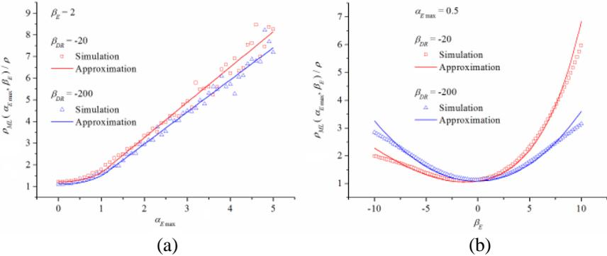
**Figure 6.** The degradation of the resolution of the multi-look SAP (a) versus  $\alpha_{E \max}$  and (b) versus  $\beta_E$ .
