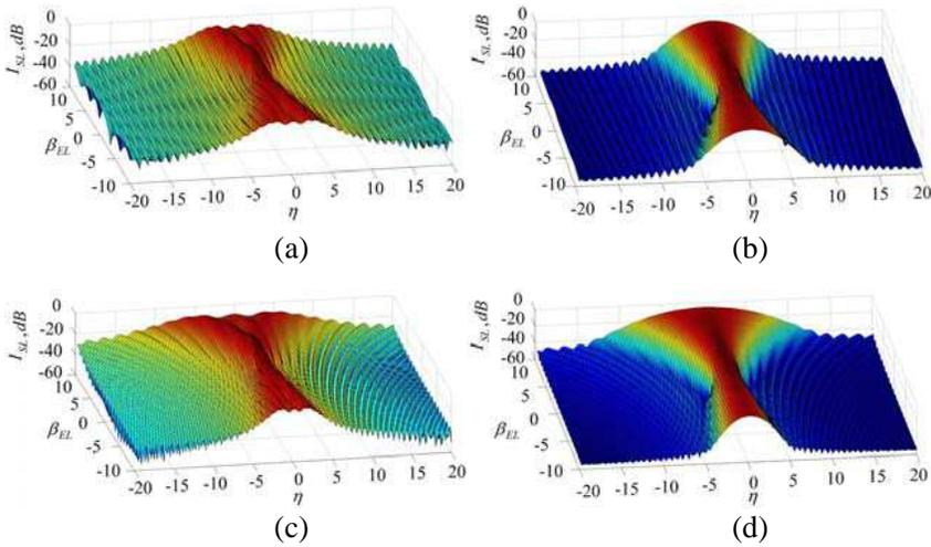
**Figure 2.** The degradation of the SAP caused by the LQPE in the cases of (a), (b) the high TBP value ( $\beta_{DR} = -200$ ) and (c), (d) the low TBP value ( $\beta_{DR} = -20$ ) for (a), (c) the rectangular window and (b), (d) the Hamming window.
