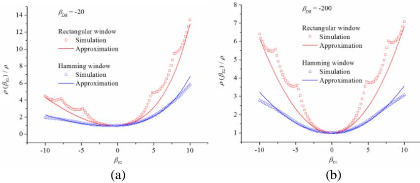
**Figure 4.** The degradation of the azimuth resolution caused by the LQPE for (a) the low TBP and (b) the high TBP values.
