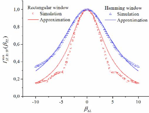
**Figure 3.** The degradation of the SAP maximum value caused by the LQPE.
