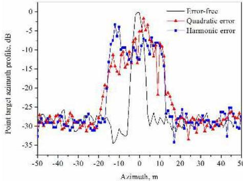
**Figure 16.** Point target azimuth profiles (taken from Figs. 13, 14(a), and 15(a), for the target indicated by the arrow).
