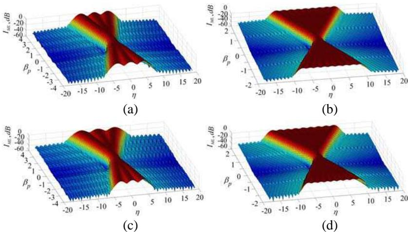
**Figure 8.** The multi-look SAPs ((a), (c) 3 looks and (b), (d) 9 looks) versus the quadratic phase error presented on the multi-look processing interval for (a), (b) a high TBP and (c), (d) low TBP.
