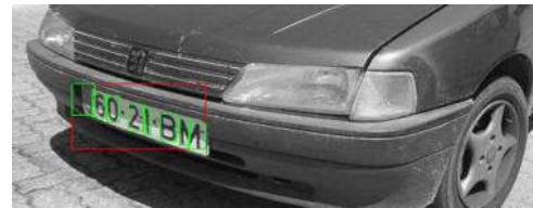
Fig. 5. Example of text detection with SWT
