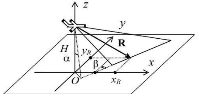
Figure 3. The antenna beam orientation angles.
