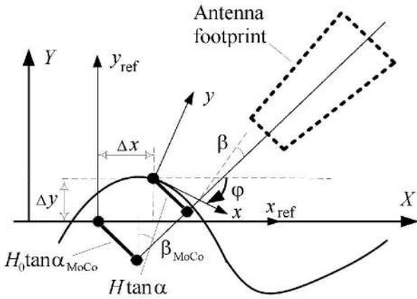
Figure 4. Flight geometry on the ground plane.
