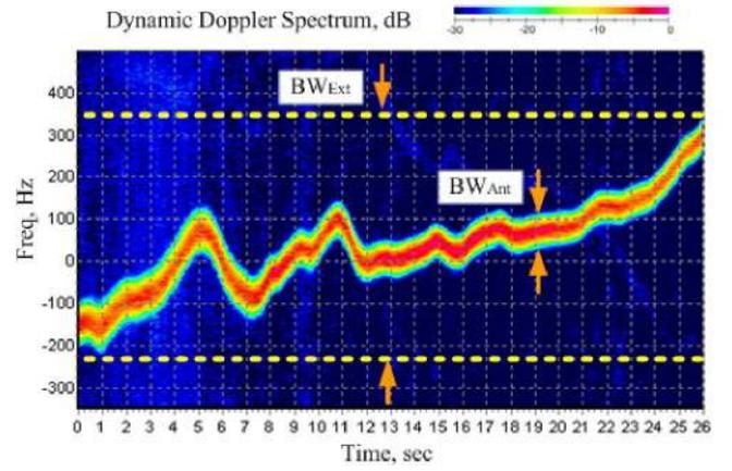
Figure 5. The dynamic Doppler spectrum of the radar data after MoCo.
