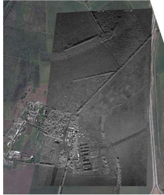
Figure 3: The 45-look SAR image formed by using the built-in geometric correction is imposed on the Google Map image of the scene.
