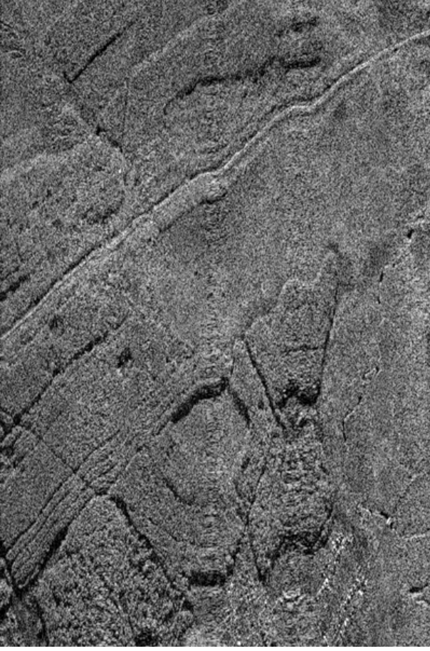
Figure 4. A single-look SAR image built with clutter lock.
