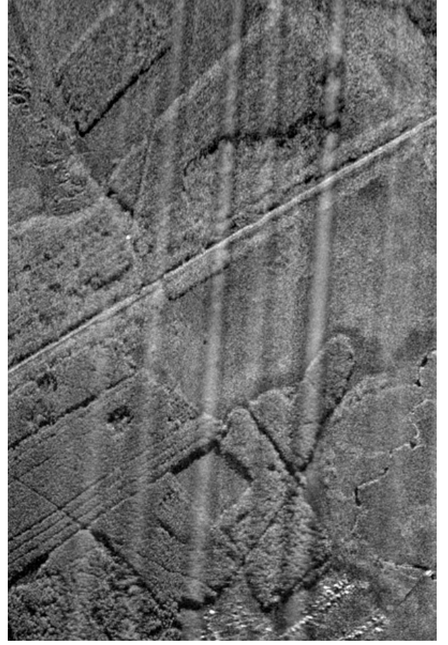
Figure 5. Multi-look SAR image built without clutter-lock by ordinary averaging of all SAR look.
