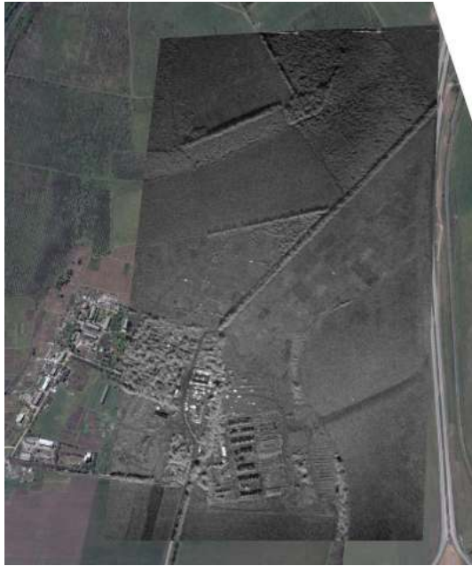
Figure 3. SAR image (45 looks) formed by using the built-in geometric correction is imposed on the Google Map image.
