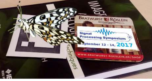
Fig. 4. Example of augmentation (left – binary marker with 3d model, right – image marker with augmented image).
