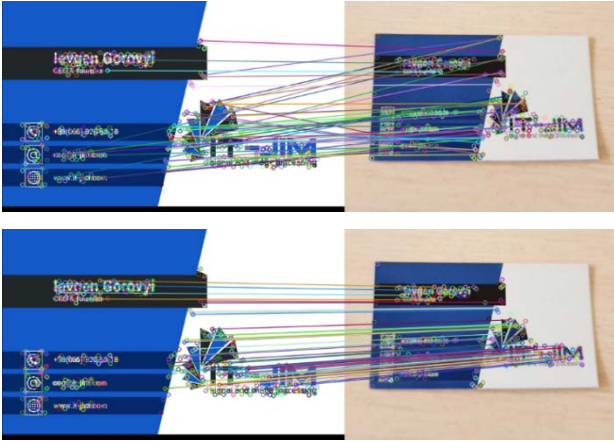
Fig. 2. Keypoint matching with ORB (upper) and AKAZE (lower).
