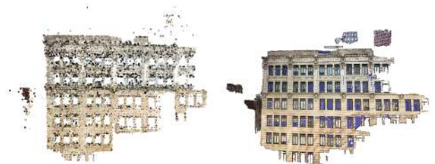
Fig. 5. MVE 3D reconstruction results for building facade: sparse point cloud and the resulting model.
